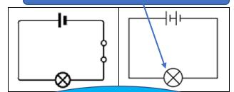
If you use a battery with a higher voltage, the bulb would also be brighter.
